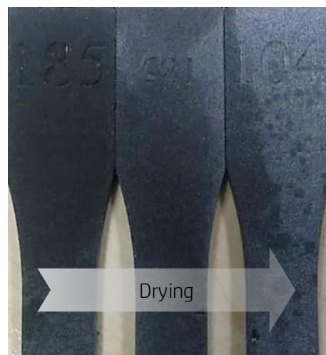
Figure 10 - Drying of brake fluid on tensiles
